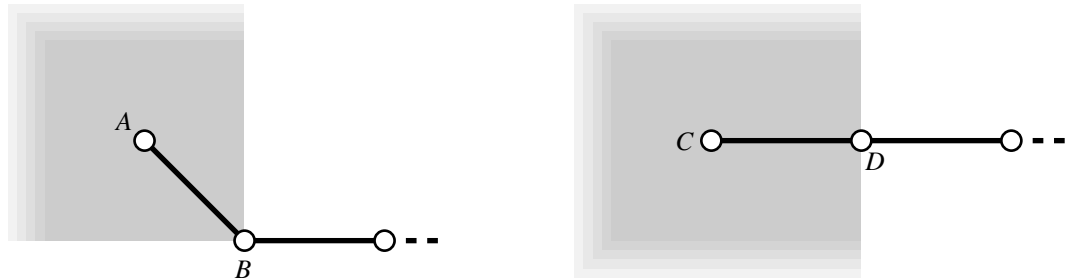
Figure 3.15: Example of the enforcement of the geographic relationships when moving a node. The grey shaded area shows the degree of freedom afforded node A (left) and node C (right).
