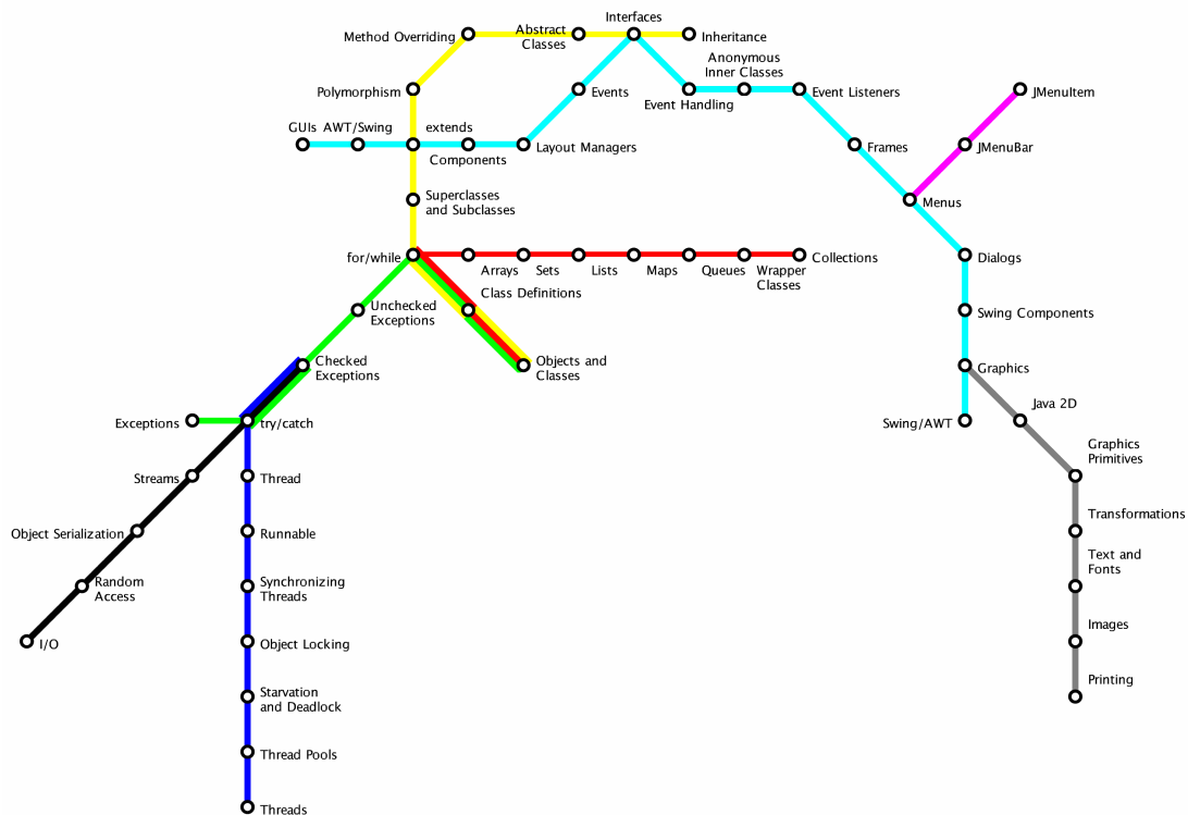
Figure 8.6: A website navigation map using the metro map metaphor using a spring embedder to produce an initial embedding. The starting point for this map is the “Objects and Classes” node in the middle.
