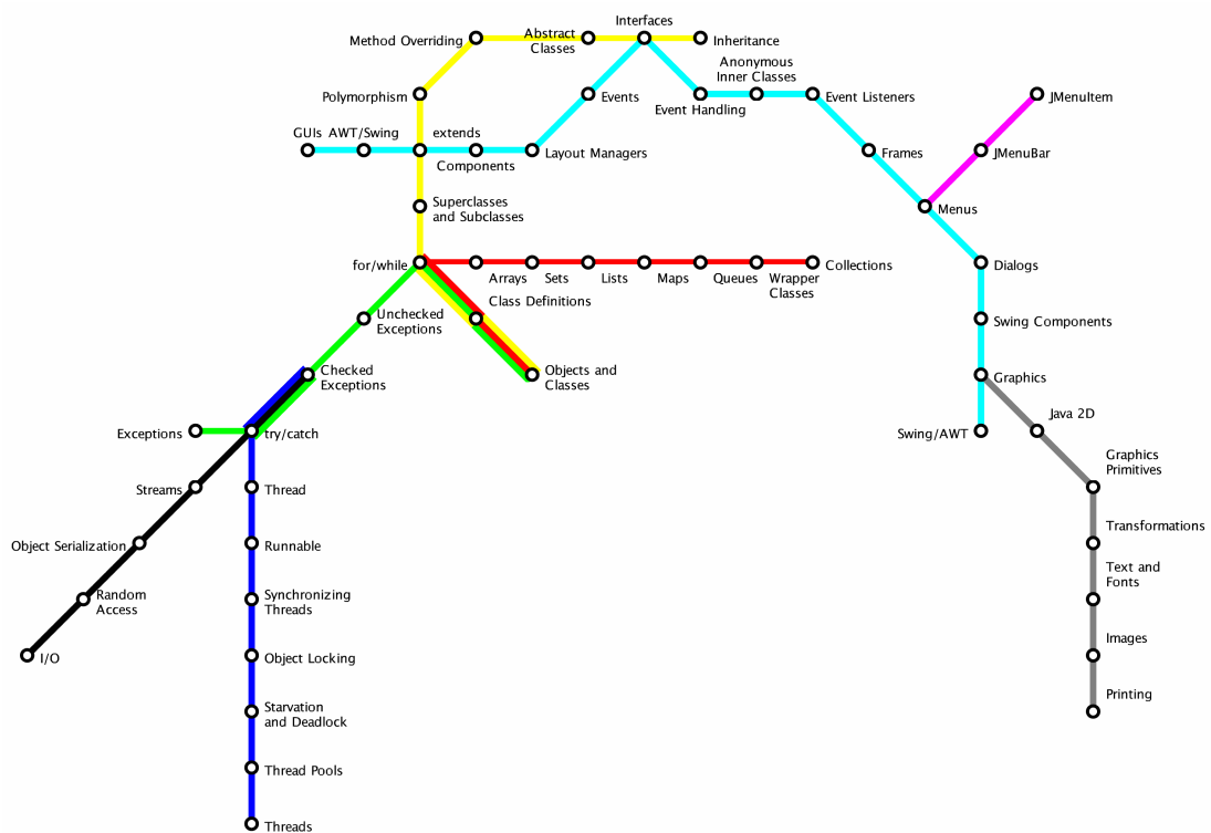
Figure 8.6: A website navigation map using the metro map metaphor using a spring embedder to produce an initial embedding. The starting point for this map is the “Objects and Classes” node in the middle.
