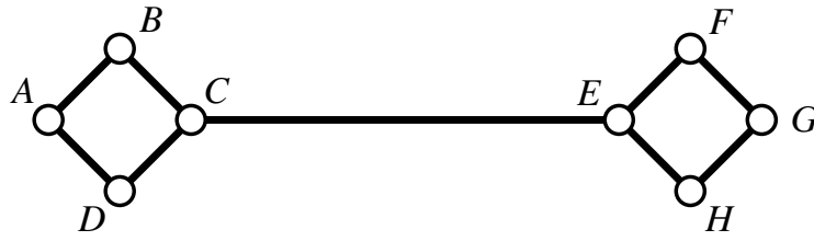
Figure 4.2: Example of clustering with a single overlenght edge. An attempt to cut the graph based on the edge CE will produce two clusters of nodes: \{A, B, C, D\} and \{E, F, G, H\}
