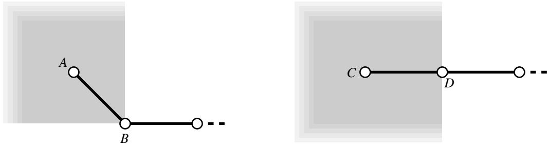
Figure 3.15: Example of the enforcement of the geographic relationships when moving a node. The grey shaded area shows the degree of freedom afforded node A (left) and node C (right).
